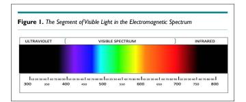
to 1 millimeter and frequency beneath 400 THz (Figure 1). The sources, as lasers, emitting light with a sole wavelength and optical frequency are monochromatic, whereas sources emitting with more than one wavelength and frequency are polychromatic, as is the sun.<sup>15</sup>
