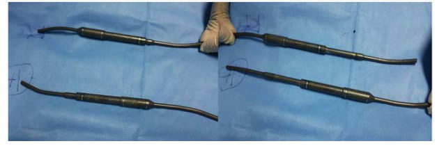
Figure 6. The MAGEC Rods Could Not Maintain Expansion and Both have Telescoping Movement, We Named that Catastrophic Failure
