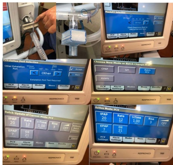
Figure 1. Add 2 HEPA Filters, One Immediately Connected to the V60 Main Gas Port Outlet and the Second HEPA Gets Connected to the Exhalation Valve Port Closer to the ET/Trach. To Connect to an ETT Tube You Need to Use the Philips Respironics Conventional Exhalation Valve and/or Circuit Kit. We Recommend that the HEPA Filter on the Exhalation Valve Port be Connected to a Blind Reservoir. Turn on Machine and Hit the Menu Tab. Please Ensure the Patient is not Connected to the V60 Machine
